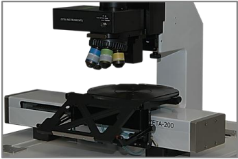
Fig. 8(a). Wafer edge measurement fixture on a Zeta-200 optical profiler.
